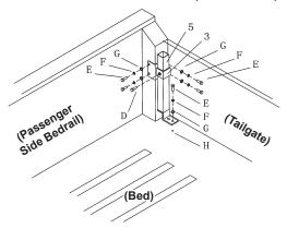
5. Attach the assembly to the Blind Fasteners as shown above using Bolts (E), Washers (F), and Spring Washers (G) - as shown above.
